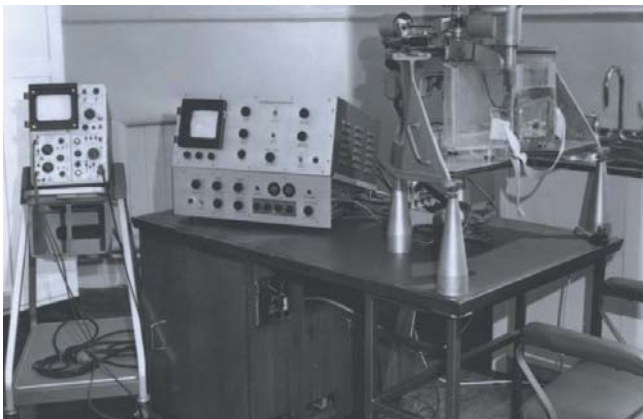
Figure 6 CAL Eye echoscope with patient coupling on the right and recording equipment on the left.
