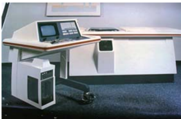
The Ausonics System 1 breast and small parts scanner which employed four 4 MHz transducers for the scanning.
