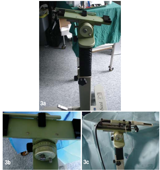
Fig. 3a: The Accuseed machine. 3b: A view from above of the Accuseed. As mentioned the probe is angled posteriorly normally approximately 12° (long arrow) while the stepper moves in 5 mm intervals (short arrow). 3c: The Accuseed with cradle and probe inserted. Water can be inserted via the tubing (long arrow) to inflate the balloon in order to lift the posterior aspect of the prostate gland above the first grid line. The plastic grid is slotted into two holes in the black retainer (short arrow).
